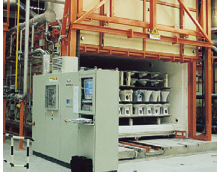
Intermittent shuttle kiln in the ceramics industry
